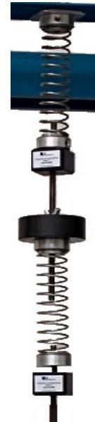
**Includes:** Three springs of different stiffness, three different weight blocks, low frequency excitation system.
