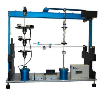
The Vibration Fundamentals Training System (alias VFT) is a turn-key integrated educational package for teaching/learning the fundamental principles of mechanical vibration as well as engineering mechanics. It provides both a comprehensive hands-on experimental device and an instrumentation package including wireless sensors for performing laboratory exercises to enhance student understanding of vibration theory.
