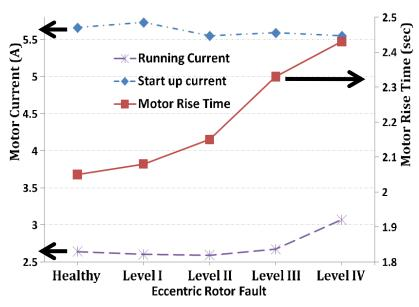
Eccentricity faults in induction motors increase motor rising time, motor slip, and motor running currents.
