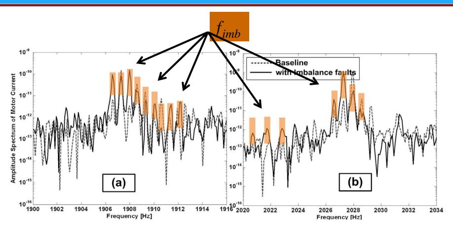
Fault components are slightly increased with mechanical imbalance faults. However, these components are observed even in the baseline spectrum showing the presence of dynamic eccentricity in the healthy motor.
