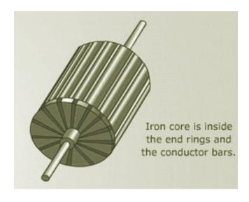
The rotor of the induction motor consists of end rings connected by the conductor bars.
