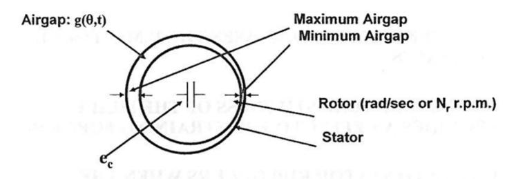
For completeness the airgap length as a function of both static (e<sub>s</sub>) and dynamic eccentricity (e<sub>d</sub>) can be expressed as:
