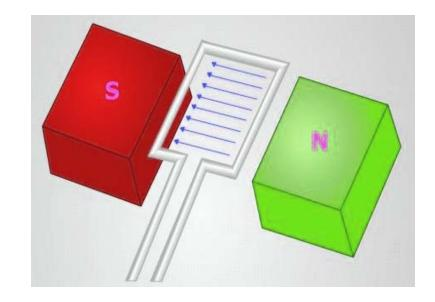
The rotor's magnetic poles at each core are attracted to opposite magnetic poles formed by the stator coils.
