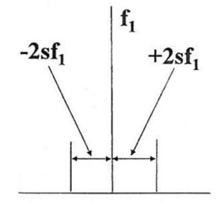
Severity is given by the amplitude difference between twice slip sidebands with line component
