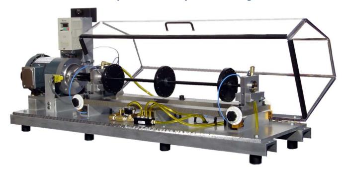
Spectra Quest's Machinery Fault & Rotor Dynamics Simulator (MFS-RDS) is an innovative tool to study the dynamic behavior for rotor supported by oil lubricated journal bearings, as well as other common machinery faults, such as balancing and resonance study. An oil pump is provided with the simulator to drive the lubrication fluid. In addition, it provides different bearing clearance selection and controllable lubrication oil pressure for rotor dynamics whirl and whip phenomena.
