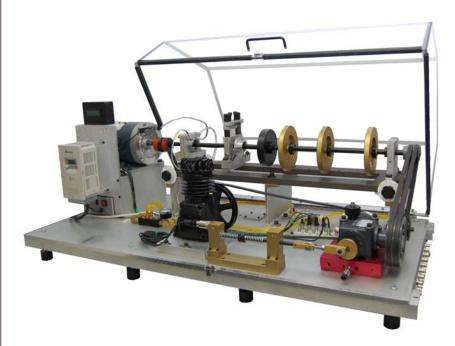
monitoring diagnosing and machinery faults before they irreversibly damage your machinery and cause breakdowns that threaten to undermine product quality, delivery and overall customer service. The success of any PdM program ultimately depends on how accurately and easily the vibration spectra, waveforms and phase relationships can be analyzed understood. Spectra and Quest's Machinery Fault Simulator Magnum (MFS-MG) is an innovative tool to study the signatures of common machinery faults without
