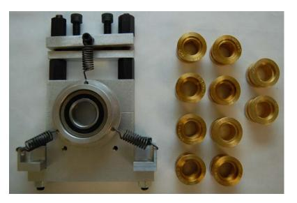
The kit consists of four sleeve bearing pairs to give bearing clearances of 2 and 6 mils (0.001') for two different lengths, two elliptical bearings to avoid whirl/whip instability, and one shaft centering device
