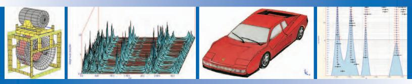
In ME'scopeVES, each point on a 3D structure model has its own local measurement axes which can be graphically oriented to coincide with the transducer measurement directions. This feature gives you the freedom to mount transducers directly on curved surfaces. Tri-axial and radial measurements are easily defined on the 3D test model using this feature.
