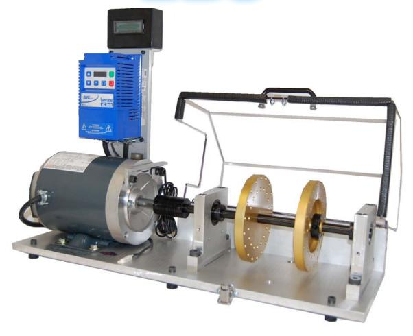
Hands-on system to study bearing faults and shaft unbalance
